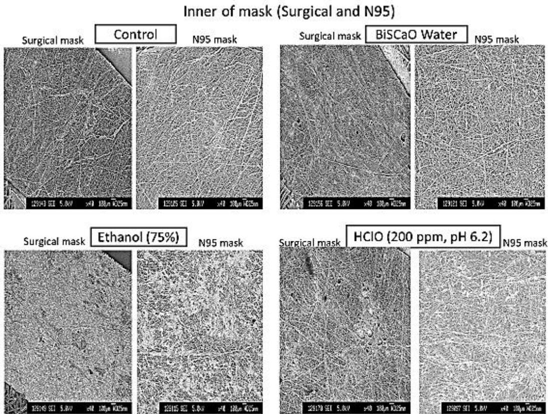
Figure 6. Non-woven fabric deterioration with BiSCaO Water, ethanol, and HClO. The SEM image of inner sheet of surgical and N95 masks, which submerged in enough amount of BiSCaO Water, ethanol, and hypochlorous acid twice per every day for 3 days.
